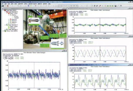
PCM-360 On-line Vibration and Condition Monitoring Software
