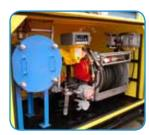
A number of aircraft refueling pumps are used to provide aircraft fuel on the airstrip. All fuel is filtered and metered to API standards for aviation.
