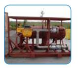
A robust pumping/filtering equipment ensures fuel is clean before the fuel reaches the Arctic  $King^{TM}$  tanks.
