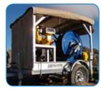
Portable fuel transfer trailers like this one enable bulk fuel transfer into tanker trucks for delivery throughout the mine.
