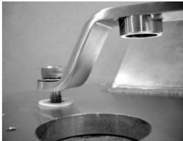
Assemble discharge cover, O-ring and spring.
