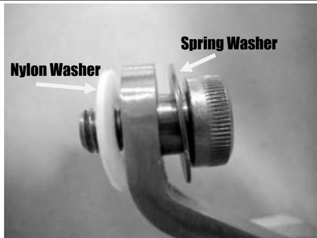
Screw shoulder bolt and handle assembly 1 to 1 ½ turns into threaded hole on door.
