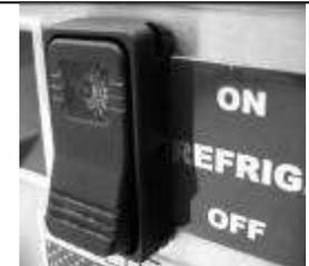
5) When the product has frozen to the desired stiffness, immediately turn OFF the refrigeration switch, and begin to discharge the product.
