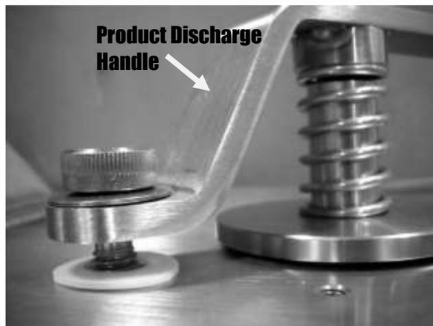
Press down on product discharge handle, ensuring the discharge cover and discharge handle are aligned with each other.
