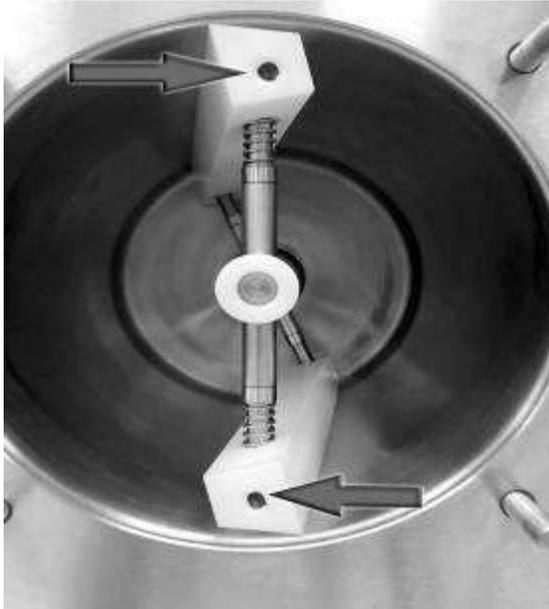
After the dasher is in place, you should be able to see the "dimple" on each of the two blades BEFORE you put the front door in place (see photo). If this is wrong the machine will not operate properly. You need to be aware of this Each and Every time you assemble the machine.
