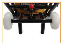
Trolley hooks into baseplate during operation
