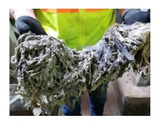
(The blockage [partially shown in the picture above] was made up of about 80% flushable wipes combined with twigs, sticks, a plastic soda bottle, feminine hygiene products, and even a pair of underwear. PHOTO CREDIT Rockland County)
