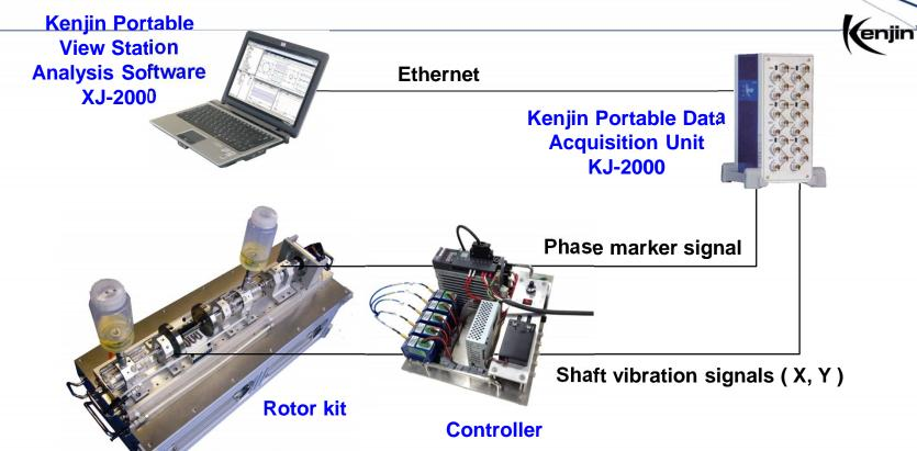
The demonstration is performed by using the rotor kit with plain bearings (journal bearings) and the Portable Vibration Analysis System "Kenjin".
