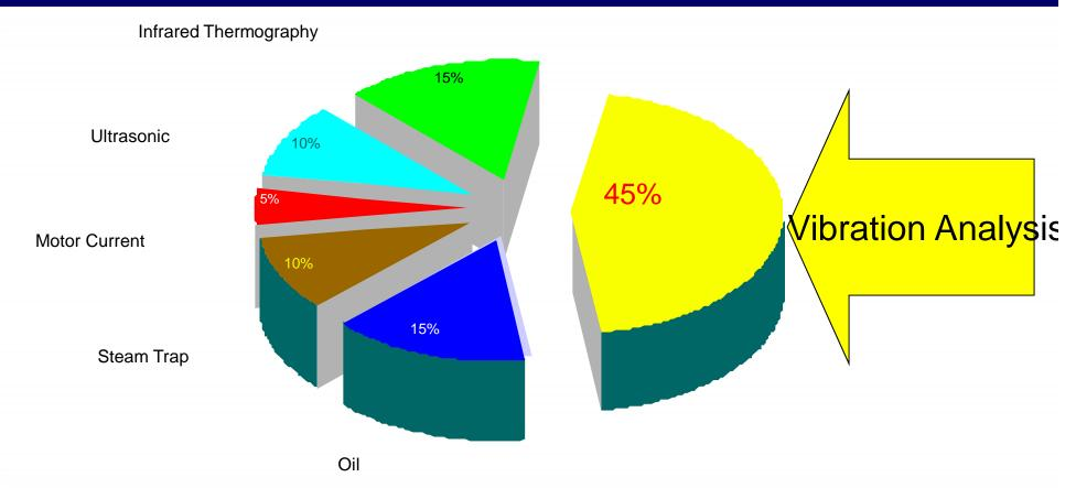
Of all the various maintenance technologies, Vibration Analysis provides the greatest percentage of payback when adopting a predictive maintenance program
