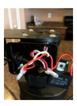
6. USING PLYERS REMOVE ONE WIRE CONNECTOR AT A TIME 7. REMOVE OLD WIRE AND FEED NEW WIRE THROUGH ASSEMBLY USING THE TWO CORD FASTENER NUTS. 8. REATTACH NEW RED & BLACK WIRE TO PROPER CONNECTION & TIGHTEN WITH WIRE SCREWS. 9. TIGHTEN SCEW NUTS TO FASTEN CORD 10. PUT ELECTRIC BOX PLATE BACK ON:
