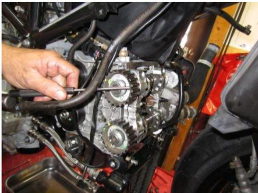
Use a punch and gently tap on the pulley to loosen the cam/cam retainers so the cam shafts can be removed.
