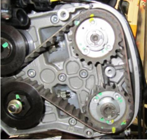
The yellow marks pictured on this horizontal cylinder are made on the pulleys where the valve cover gasket sets on the cylinder head. The three previous pictures show the pulley alignment at the “home” position. The markings will be necessary for reassembly when the belts have to be removed for shim (or belt) changing.
