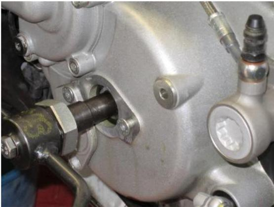
Once the spark plugs are removed, the engine turning tool can be installed. Remove the cover on the left side of the engine and install the engine turning tool onto the end of the crankshaft. Note: the tangs on the engine turning tool fit neatly into indents on the crank shaft. Tighten the bolt to snug and the engine is ready to turn counter clockwise (CCW) into the correct position(s) for valve clearance checking.
