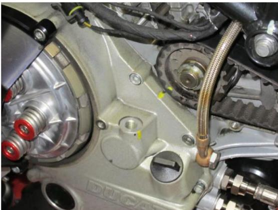
With the belt covers removed check alignment on the belts and pulleys. The intermediate shaft drives the cam belts. There is a mark (dimple) on the pulley and a mark on the engine case. At TDC of the horizontal cylinder, the marks will align. Use the paint pen to mark this alignment. Slight rotation of the engine forward/back may be necessary to locate TDC at this point.
