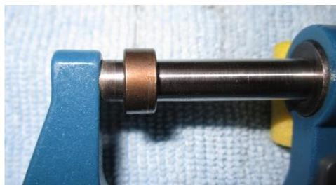
Close the micrometer. Do not over tighten. Press the "zero" button to set the reading to 0.00. Open the micrometer and place the shim on the stationary shaft of the micrometer, with the flat side towards the fixed portion of the micrometer. Measure the opening shim and record the measurement in column D of the worksheet. Determine the size of the replacement shim by adding column C to column D and record this number in column E. The number in column E is the ideal shim size to
