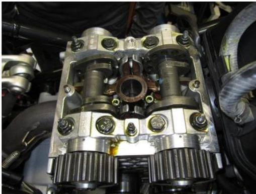
When removing the cam hold-down clamps loosen the inner and then the outer retaining nuts. These nuts are  $\frac{1}{2}$  the normal height and it is best to use a 6pt socket.
