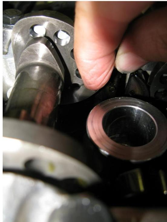
Use a feeler gauge (A), to measure the clearance between the opening rocker arm and the lower edge of the camshaft lobe: Use progressively larger/smaller feeler gauges until the size of the clearance can be determined. The proper feel is if the resistance on the feeler gauge is similar to inserting the gauge into a large book. Once the clearance is determined, record this as measurement “A” on the worksheet.
