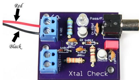
Photo # 1 Connecting power to the tester
