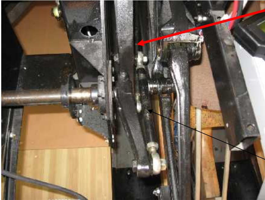
and the 2 short sweep rod jam nuts, (getting about 12-14 threads showing (total)- combining the threads showing on both sides of the long rods beyond the snug jam nuts, for equal "hang" position at zero degrees across the center) make sure that female half of telescoping tube is screwed-in tight against the
