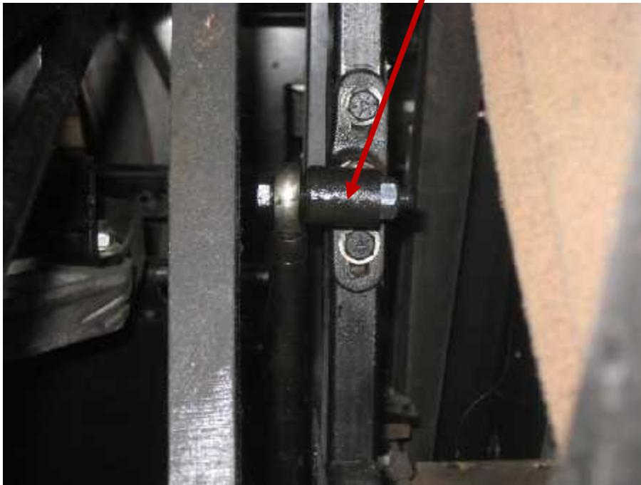
Turn the Threaded Link LONGER to raise the height at Guard Position, or make the Threaded Link SHORTER to LOWER the sweep height at Guard Position. Make sure that the Threaded Link is parallel to the lane after retightening.
