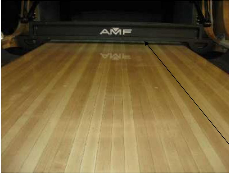
2. Adjust first guard height over lane with threaded link (to about 1.25" off lane),
