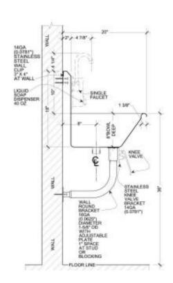
Engineering Specification: 14 gauge, type 304 stainless steel wash sink.1-3/8" rolled rim. 1-1/2" welded in drain. Exposed surfaces polished to a satin finish. Supported on (2) wall clips.
