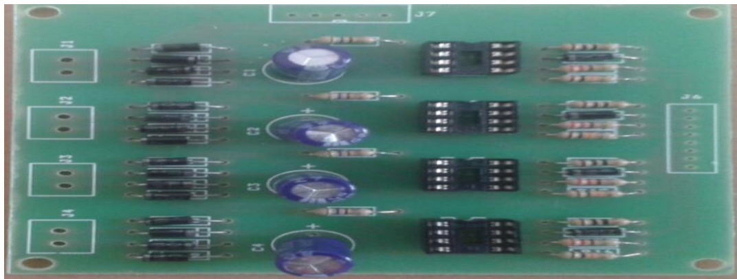
Fig. 11. Isolator and Driver Circuit
