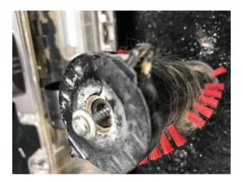
12. Pull off end cap and remove the hair and debris that may have accumulated there.
