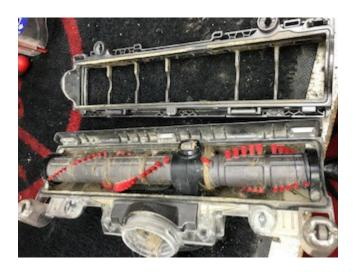
5. Use Phillips #1 to remove four screws holding roller brushes.
