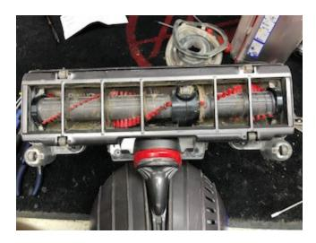
2. Use flat head screwdriver to gently pry red clip up and off completely.
