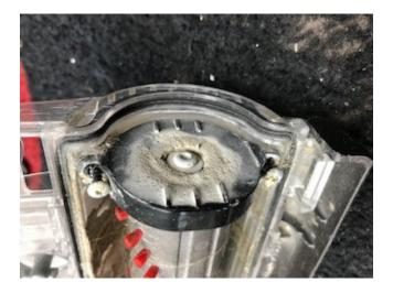
6. Pull one roller out of gear box.
