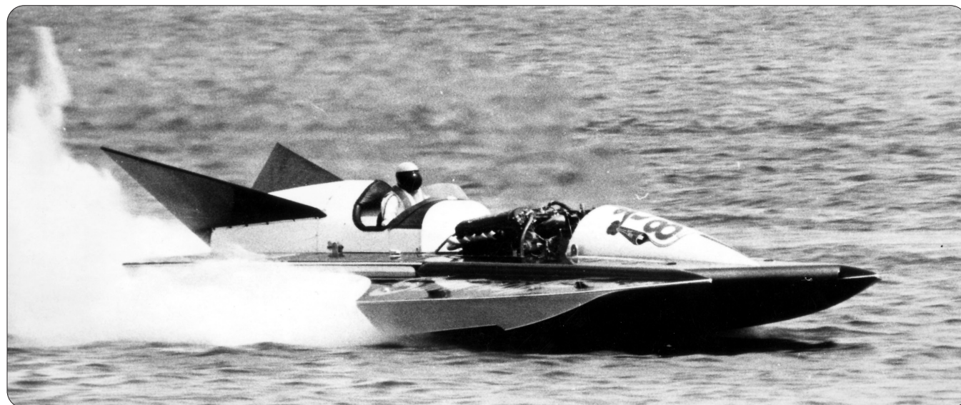
TOP: The Schoenith team introduced a radical step-hull named Gale's Roostertail in 1967. ABOVE: In 1968, the team introduced another radical design with a Smirnoff boat that attempted many new aerodynamic ideas to make it safer. Unfortunately, it was also too heavy to be competitive.
