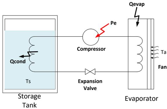
**Figure 2.** The heat pump system using ambient air
