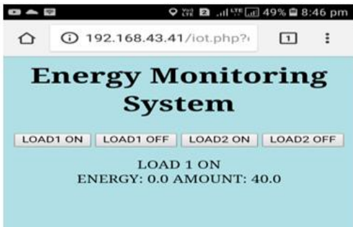
Figure 3.1: WSN Energy monitoring system
