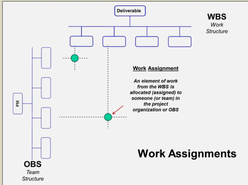
In practice such drawings as the above are used for communicating the concept of work assignment for education purposes only and the real work assignments are captured in a matrix.
