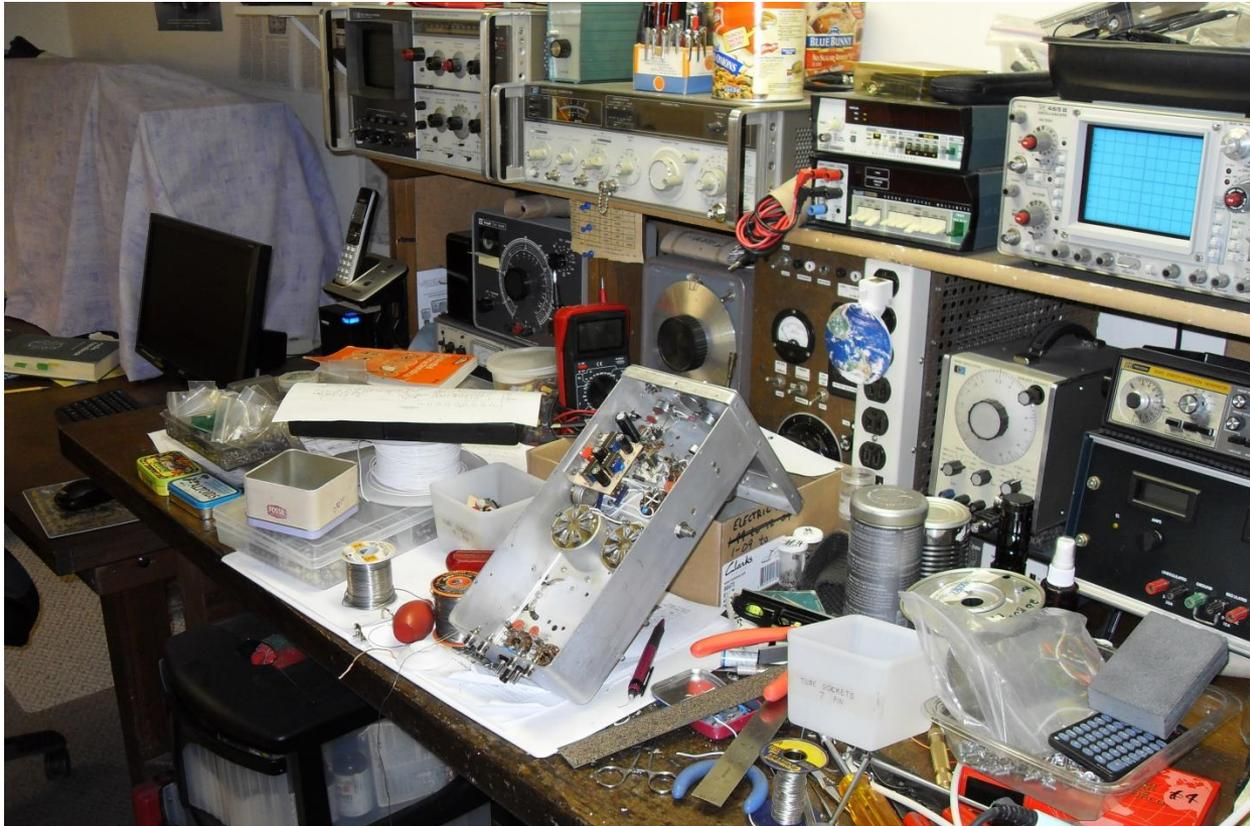
The 80m Cheap 'N Easy II in the middle of the wiring phase. I always use silver coated, stranded teflon wire, and zip tie it into bundles as required after completion. I find that I have to stop and clean up the bench every so often just so I can find stuff!
