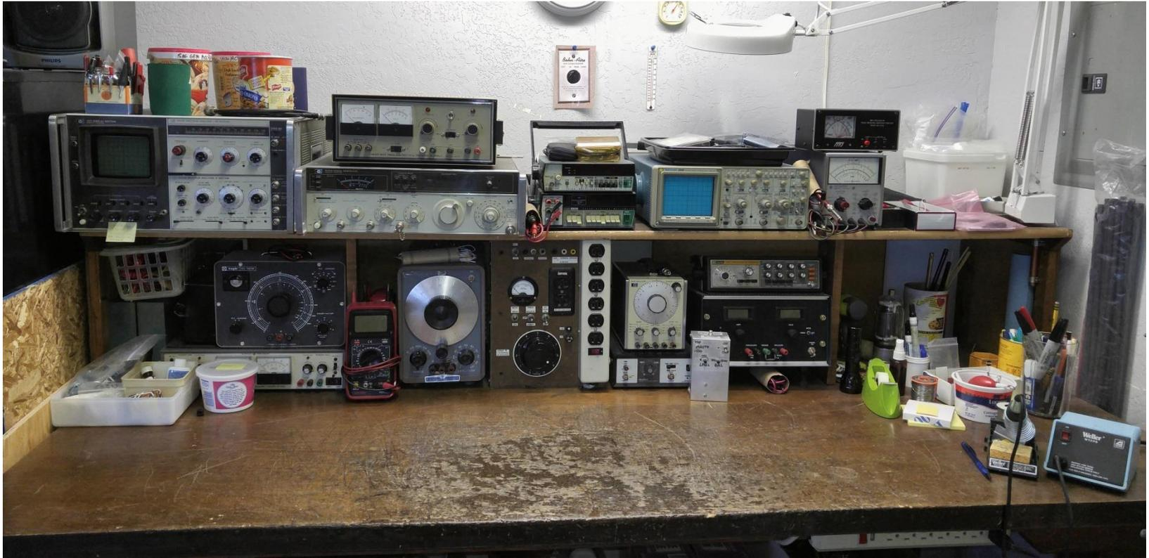
Decent test equipment really helps. For an SSB transmitter, essential are a wideband scope, two-tone audio oscillator and spectrum analyzer. For a receiver a good signal generator is a must. You need a frequency counter for either. The Heathkit lab power supply is useful for breadboard and element testing.
