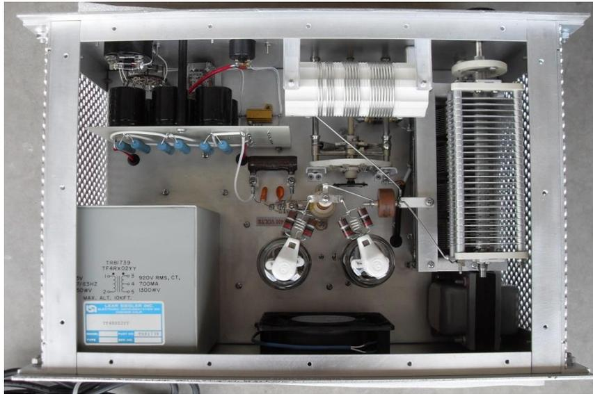
Voltage doubler delivers about 2,700 VDC no load. PA coil is wound on a form from a TU-5 unit. Bandswitch is heavy duty unit made by Radio Switch Corp. Plate transformer was a NOS military unit from Surplus Sales, but they are now out of stock.
