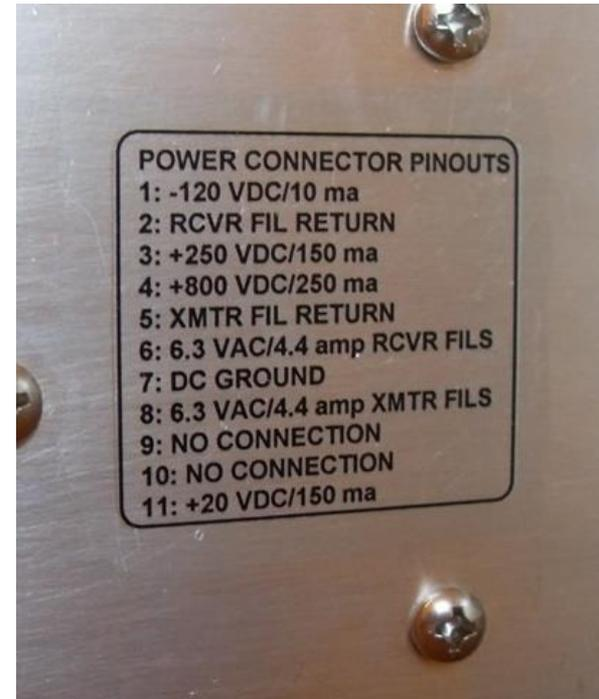
These labels were made with water slide decals printed on Papilio stock with an HP laser printer. The labels were designed using Microsoft Visio software. The front panel was oversprayed with clear matte finish from a rattle can. The chassis label was brushed with polyurethane semi-gloss.
