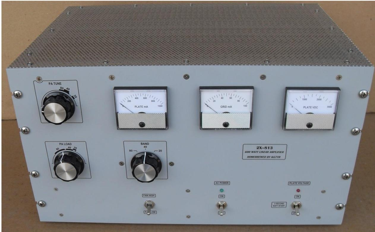
This linear was built to go with the Octal Tri-Bander. I always liked the look and feel of an 813. This amplifier uses a pair of them in grounded grid. A lot of the design is similar to my HB-600 linear. NOS Triplet meters monitor grid mA, plate mA, and plate VDC.
