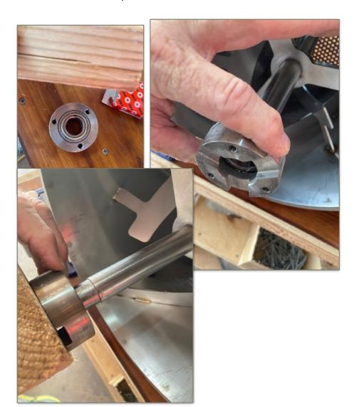
8.Remove and inspect to ensure bearing and holder are flush against front plate of drum of roaster (front plate not shown in this illustration as we are just doing a demo on a spare drum)
