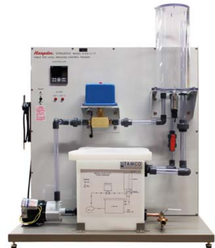
MODEL H-ICS-LT-TT Level Process Control Trainer
