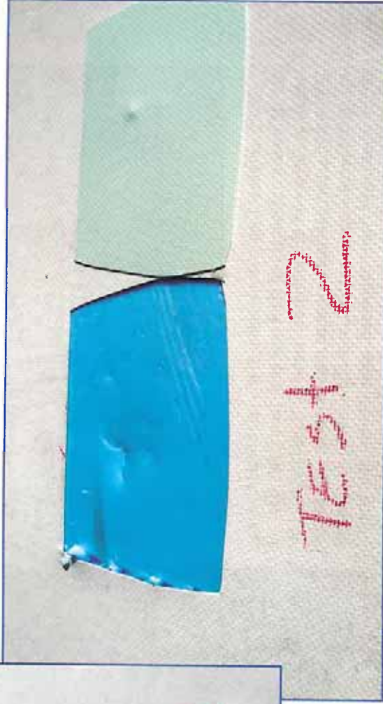
Photo 35 – Large depression in insulation board.
