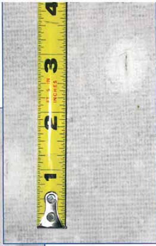
Below: Photo 6: - Spiral and linear fractures in single- ply membrane.
