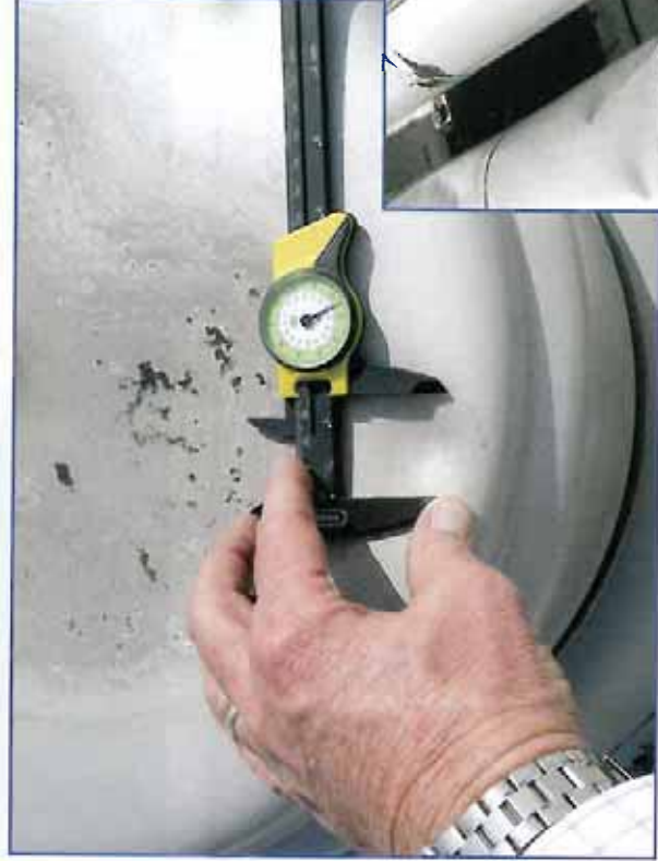
Photo 18 – Dents in metal equipment hood. (5)
