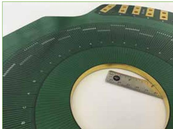
FIGURE 2. Circuit Connect applies its PCB knowledge to non-PCB products, such as this 0.320" heavy copper product with solder mask and gold edge plating ...
