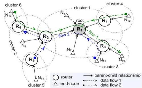
Fig.4: Cluster-tree topology with 2 time-bounded data flows
