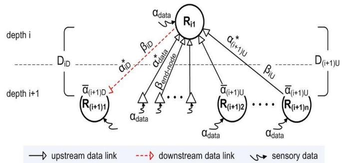
Fig.6: General data flow model with corresponding arrival and service curves.
