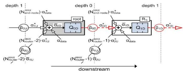
Fig.8: The queuing system model for downstream direction.
