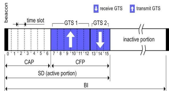
Fig.2: Super frame structure of IEEE 802.15.4.
