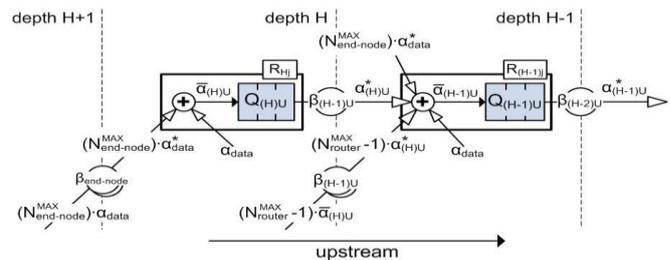
Fig.7: The queuing system model for the upstream direction
