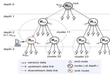
Fig.5: The worst-case cluster-tree topology model corresponding to a configuration where  $N^{MAX}$  end-node = 3,  $N^{MAX}$  router = 2,  $H_{sink} = 2$  and  $H = 2$ .
