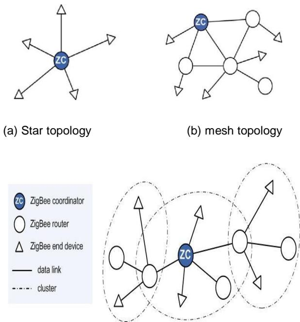
Fig.3: IEEE 802.15.4/Zigbee network topologies
