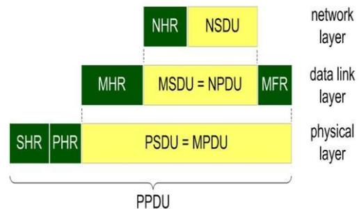
Fig.1: Structure of the IEEE 802.15.4/Zigbee frames
