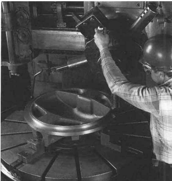
Cast domed disc being machined.
