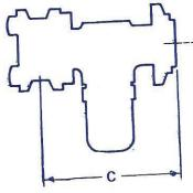
SIZES 1" THRU 4" HAVE 4 BOLT SQUARE FLANGES SIZES 5" THRU 8" HAVE ROUND FLANGES
