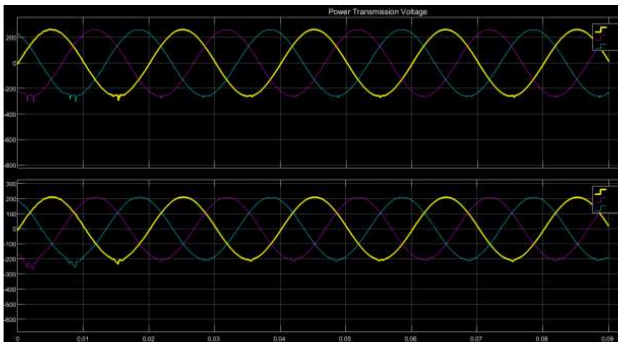
Fig.9 The output power transmission voltage of the system model with UPFC
