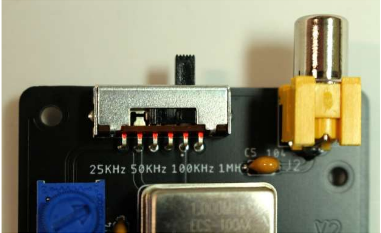
Selector Switch and Output Jack - Switch in the 1 MHz position
