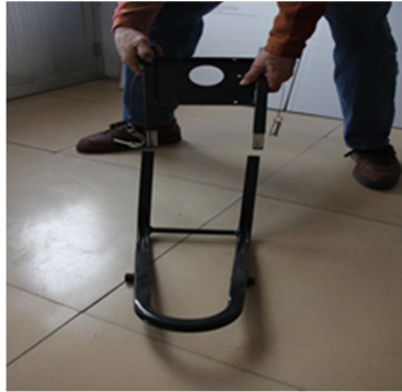
1. Put together upper and lower main frame. Do not put in bolts.
