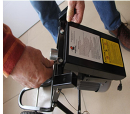
6. Install metal cover on gear motor with 5/16x3/4 bolts.
