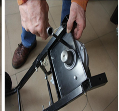
5. Install gear motor with flat washer, spring washer and nuts Tighten
