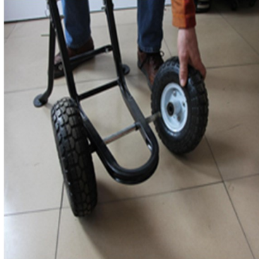
4. Install wheels and axle. Put on washer and cotter pin. with 10 MM wrench..
