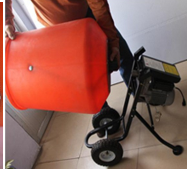
8. Slide on drum. Line up 1/2" hole.
