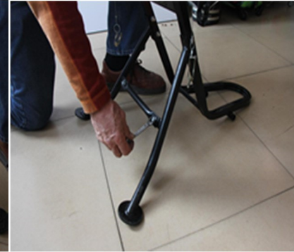
3. Install leg brace using 5/16x3/4 bolts and 5/16 nuts.
