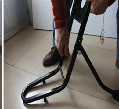
2. Install legs with 5/16x1-1/4 bolts and 5/16 Nuts.
