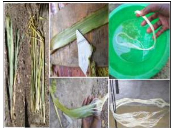
Figure 2. Pineapple leaf fiber extraction by scrapping method
