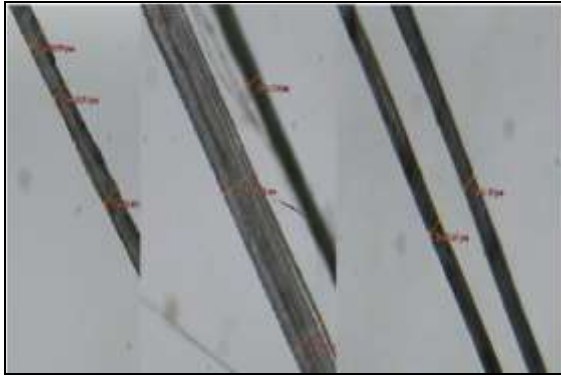
Figure 7. Longitudinal structure of pineapple leaf fiber under leica microscope
