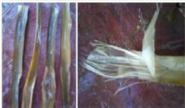
Figure 3. Pineapple leaf fiber extraction by retting methods
