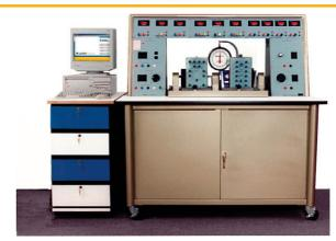
The Hampden Model HMD-100-CM-DA-CDL Mobile Console provides the facilities required to perform experiments with Series 100 Motors and Generators plus power and metering services. The Student Experimentation Station allows experiment values and test results to be directly fed into typical PC data acquisition boards (not included), such as Data Translations, Analog Devices and Metrabyte.
