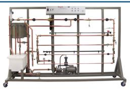
The Hampden **Model H-6925-CDL** Fluid Circuit Demonstrator provides complete facilities for the investigation of the phenomena associated with incompressible fluid flow in conduits. The analog outputs are
