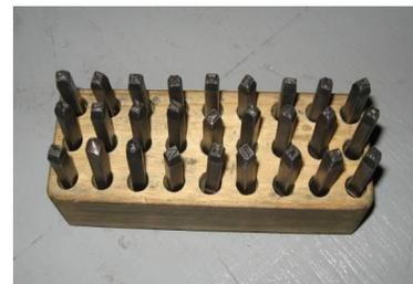
N.B. It is important to never punch parts that have been hardened, plated or anodized.
