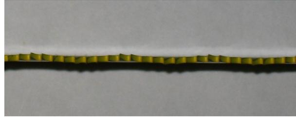
reduces friction but makes the blade difficult to control and keep cutting straight. This is why precision hacksaw blades have no offset. It is the difference between the blade set and body height that defines the smallest possible radius that can be produced with a given blade.
