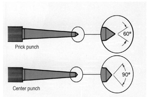
For drills that are 1/4" or smaller, the drill can be started directly in the indentations. A centre or spot drill will be used before using drills larger than 1/4".
