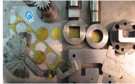
It is important to remember that mass producing parts requires specialized tooling (moulds, punch and dies, fixtures ...) that need to be produced by very competent machinist, toolmakers, mould makers ... These specialized tools are often produced in tool rooms using traditional or CNC machines.
