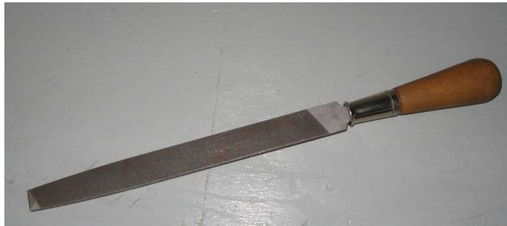
A file's surface is made up of a large number of teeth. These teeth incorporate a cutting surface and cutting lips that will engage with the part and produce chips by plastic deformation. Files are unidirectional cutting tools, they cut from the tip of the file to the handle and no pressure should be applied on the backstroke.
