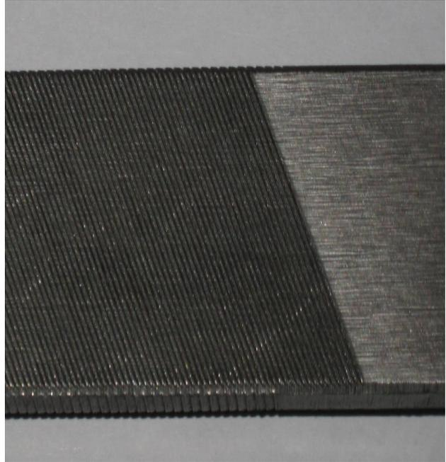
**DOUBLE CUT FILES** have diamond shaped teeth that are the result of two intersecting rows of teeth similar to the single cut ones. This tooth form is generally used for roughing cut since the smaller contact area permits better penetration so they can take deeper cuts. The space between the teeth also permits for more chip clearance which is helpful when filing large surfaces.
