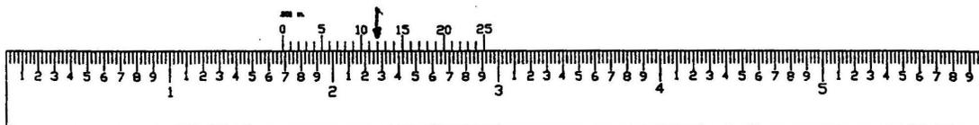
A metric vernier calliper also has two scales the longest is the fixed scale and it is graduated in 1 mm segments every tenth segment representing 1 cm.
