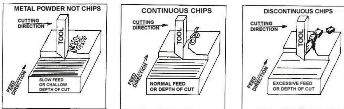
**N.B.** The feed is the most important variable for surface finish (but not the only one).
