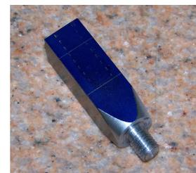
To avoid flaking and in order to produce fine and accurate lines it is important to apply only the finest of coats and to do so on a very clean (degreased) surface.
