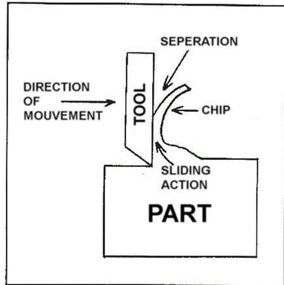
The **interior surface** of the chip results from the compression of material since it never comes in contact with the tool. It is the least relaxed surface of the chip and that means that it pulls on itself (tension). The interior surface of the chip has a rough and a mat finish and an internally curved surface.
