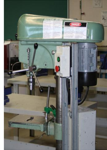
**Thin parts:** Sandwich thin parts between thicker parts of a similar material or *assemble a support drill jig* directly on the work table.
