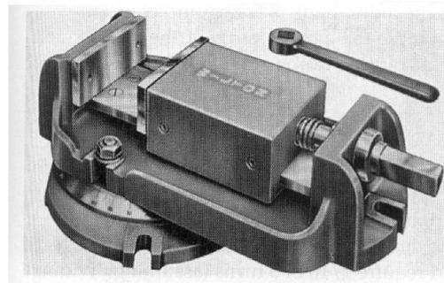
Some machine vices incorporate a rotary base (for angular cuts) and or a pivot axis (for compound cuts). Rotary base vices and universal vices should only be used when required since the rotary axes reduce rigidity and make for a weaker setup.
