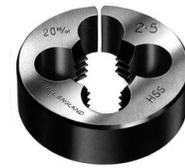
**TWO PIECE ADJUSTABLE DIES** (or adjustable dies) are used for progressive cuts in tough materials or for large (deep) threads. Since the two die halves are adjustable, several roughing passes can be taken, thus reducing the force required for each pass and also reducing the possibility of tearing the thread. They can also be used to rough out threads that will be finished with a solid or split die.
