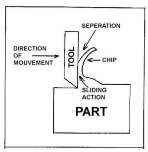
The **interior surface** of the chip results from the compression of material since it never comes in contact with the tool. It is the least relaxed surface of the chip and that means that it pulls on itself (tension). The interior surface of the chip has a rough and a mat finish and an internally curved surface.
