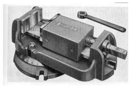
N.B. Although one could use a dead blow hammer to loosen a machine vice's handle, it should never be used to tighten one. The vice handle has been designed for the vice and handle extensions should not be used so if the vice is having trouble holding the part get a bigger vice!
