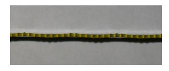
reduces friction but makes the blade difficult to control and keep cutting straight. This is why precision hacksaw blades have no offset. It is the difference between the blade set and body height that defines the smallest possible radius that can be produced with a given blade.
