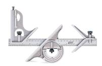
combination set is a very versatile tool used to guide the scriber during layout.
