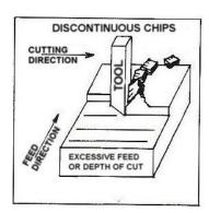
**N.B.** The feed is the most important variable for surface finish (but not the only one).
