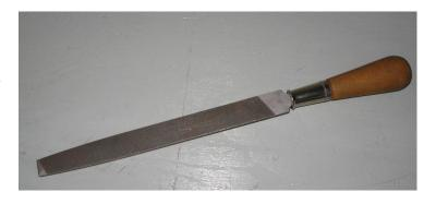
A file's surface is made up of a large number of teeth. These teeth incorporate a cutting surface and cutting lips that will engage with the part and produce chips by plastic deformation. Files are unidirectional cutting tools, they cut from the tip of the file to the handle and no pressure should be applied on the backstroke.
