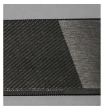
bouble Cut files have diamond shaped teeth that are the result of two intersecting rows of teeth similar to the single cut ones. This tooth form is generally used for roughing cut since the smaller contact area permits better penetration so they can take deeper cuts. The space between the teeth also permits for more chip clearance which is helpful when filing large surfaces.
