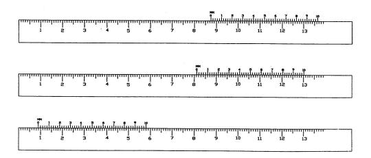
Associate dimensions with scales: 0.006" 81,18mm 87,46mm 0.304" 8,94mm 4.023" remember that the lines on an actual vernier scale are much crisper than these scans.
