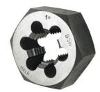
**SPLIT DIES** are slightly adjustable and are used to cut class 1, 2 or 3 threads in readily machinable material. They are also often used to finish threads roughed out on the lathe in tough materials. The slight adjustment permits one roughing and one finishing cut.
