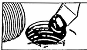
Step 5) Fill damage with FORM-A-THREAD™ compound.
