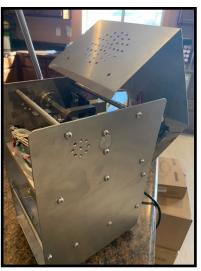
Adjust Handle to proper position while you push down on spring bracket
