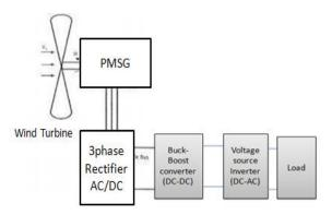
Fig 2: Proposed PMSG based WGS system
