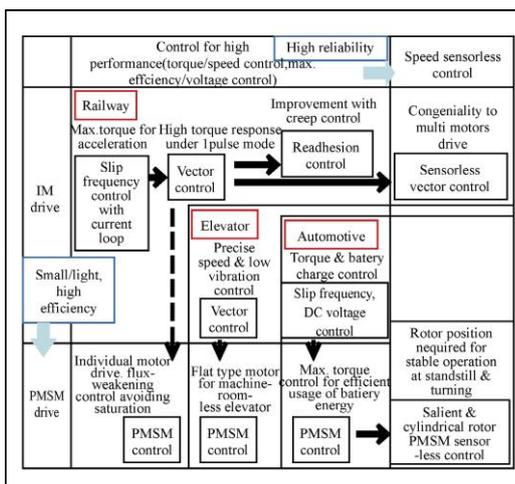
Table 2 describes some issues for advancement of AC motor drive technologies for spreading many applications. It will be shown as follows; Ultra- high speed drives, low speed and high-accuracy drives by sensorless control, large capacity drives fed by multilevel inverter, ultra-small size motor, high response and torque accuracy, downsizing and efficiency, standardization, and so on.
