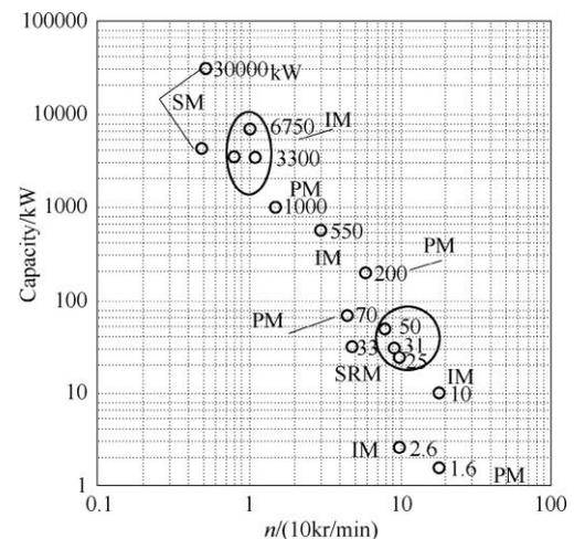
Fig.5 Nominal output power versus rotation speed of some of the prototyped and or manufactured high speed machines
