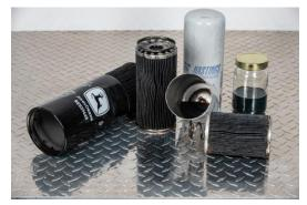
(Year Round issue). There is an ongoing epidemic of excessive diesel fuel filter changes due to today's High Pressure Common Rail (HPCR) & Electronic Fuel Injection Systems. Rail pressures in HPCR fuel systems are ranging from 5,000 psi to over 29,000-50,000 psi. Tolerances are millionths of an inch and fuel contamination is not tolerated.
