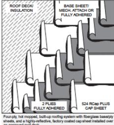
Four-ply, hot mopped, built-up roofing system with flangeless baseply sheets, and a highly-reflective, factory coated cap sheet installed over an approved roof deck.
