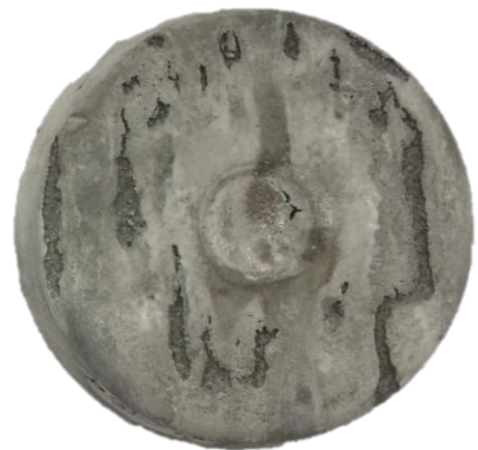
Anode Sample After 14 day Mass Loss Method Test
