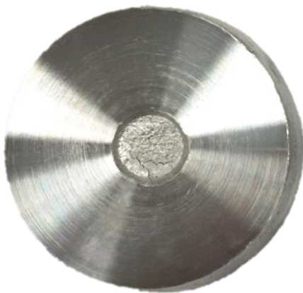
Anode Sample Before 14 day Mass Loss Method Test
