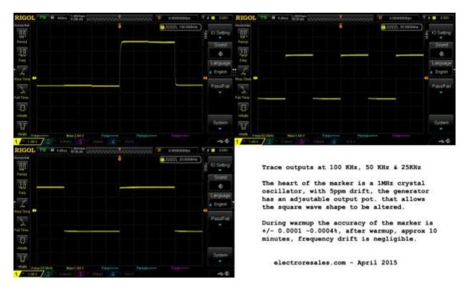
To use with a radio for actual calibration, the signal from the calibrator RCA jack needs to be coupled to the radio under test, this can be directly to the antenna jack or a looser coupling can be achieved with placing the output lead near the radio LO. Some experimentation may be required, but remember;
