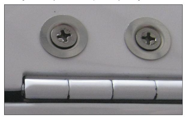
Figure 1. Hinge pin captured by tail skin. Acceptable.
