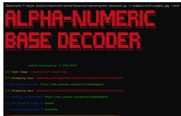
Output Fig 2: It takes an image as an input and decodes and shows the message hidden in its Exif data..
