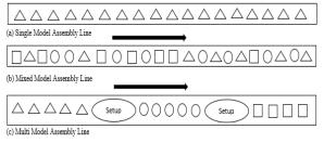
Figure 4: Assembly lines for single and multiple products **iii). Multi-Model:** In this model the uniformity of the assembled products and the production system is not that much sufficient to accept the enabling of the product and the production levels [7]. To reduce the time and money this assembly is arranged in batches, and this allows the short term lot-sizing issues which made in groups of the
