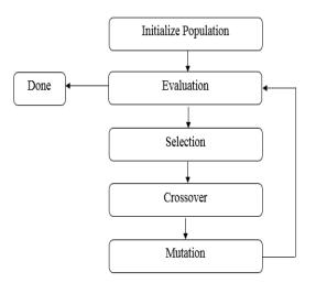
Figure 6: Flow chart of genetic algorithm Flow chart 2
