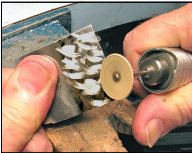
Making slash texture with the sandpaper toward the operator.
