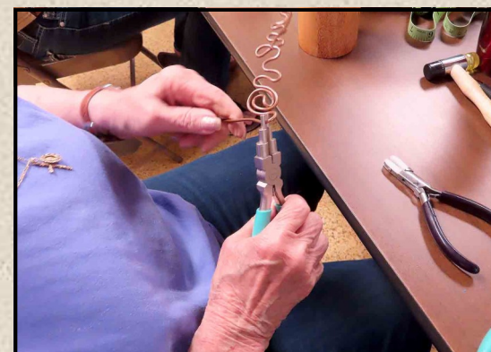
Bending heavy copper wire with wire forming pliers
