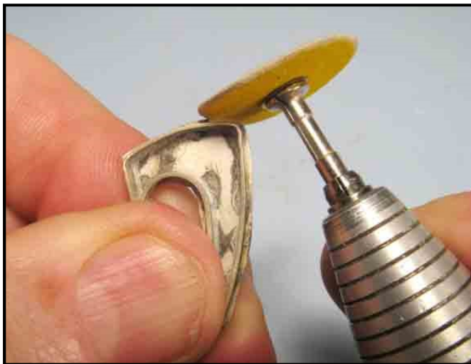
Grit side facing away from the operator.
