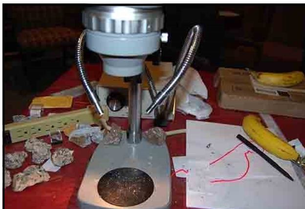
Microscope with twin directed lamps to give even light across the selected specimen.
