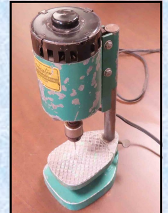
Rovie's automatic drill. The chuck moves up and down automatically as the bit turns.
