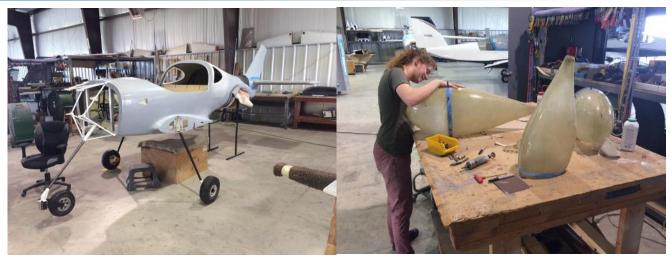
The Turbine Lightning Taking Shape - Hanna Working on Wheel Pants
