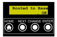
The last message shows how the Echo is routed. The default is "Base". This indicates that the Echo will be transmitting directly to the base.
