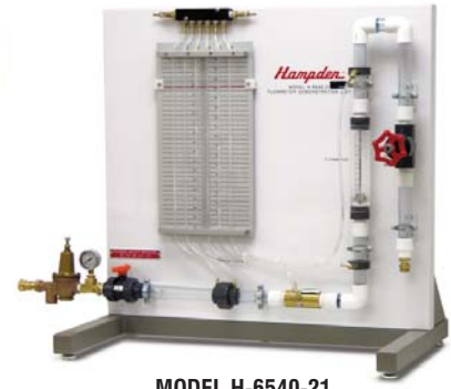
MODEL H-6540-21 Flowmeter Demonstrator Module Dimensions: 36"H x 36"W x 22"D Shipping Weight: 236 lbs.
