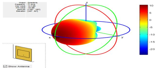
Fig.3: D pattern of patch antenna
