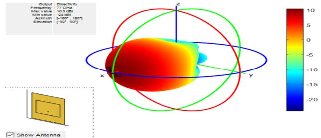
Fig.3: D pattern of patch antenna
