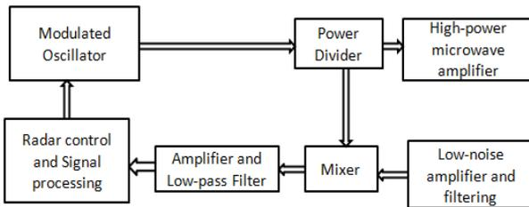
Fig.1: FMCW Radar
