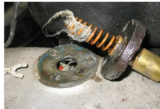
Debris accumulated on magneto contact. (Photo compliments of Steve Jelf, Parkerfield, KS.)
