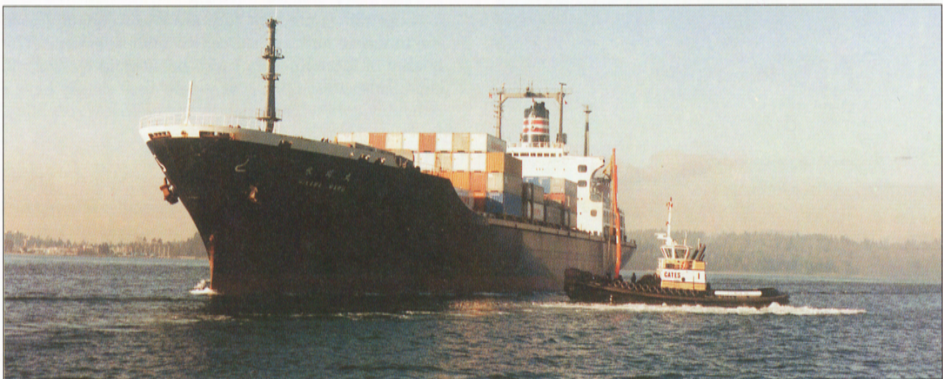
Figure 7.25 Reverse tractor tug 'Charles H Cates 1' (l.o.a. 22.5m, beam 8.5m, bollard pull ahead 38 tons, astern 32 tons) with line handling crane
